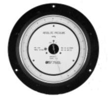
For most routine test and production uses, this capsule-type gauge offers an acceptable balance among size, readability, accuracy, and price. Available in nine standard ranges, the Series 300 is convenient to use. Absolute pressure is applied to the case and readout is direct without barometric correction. Readings are referenced to zero absolute.
